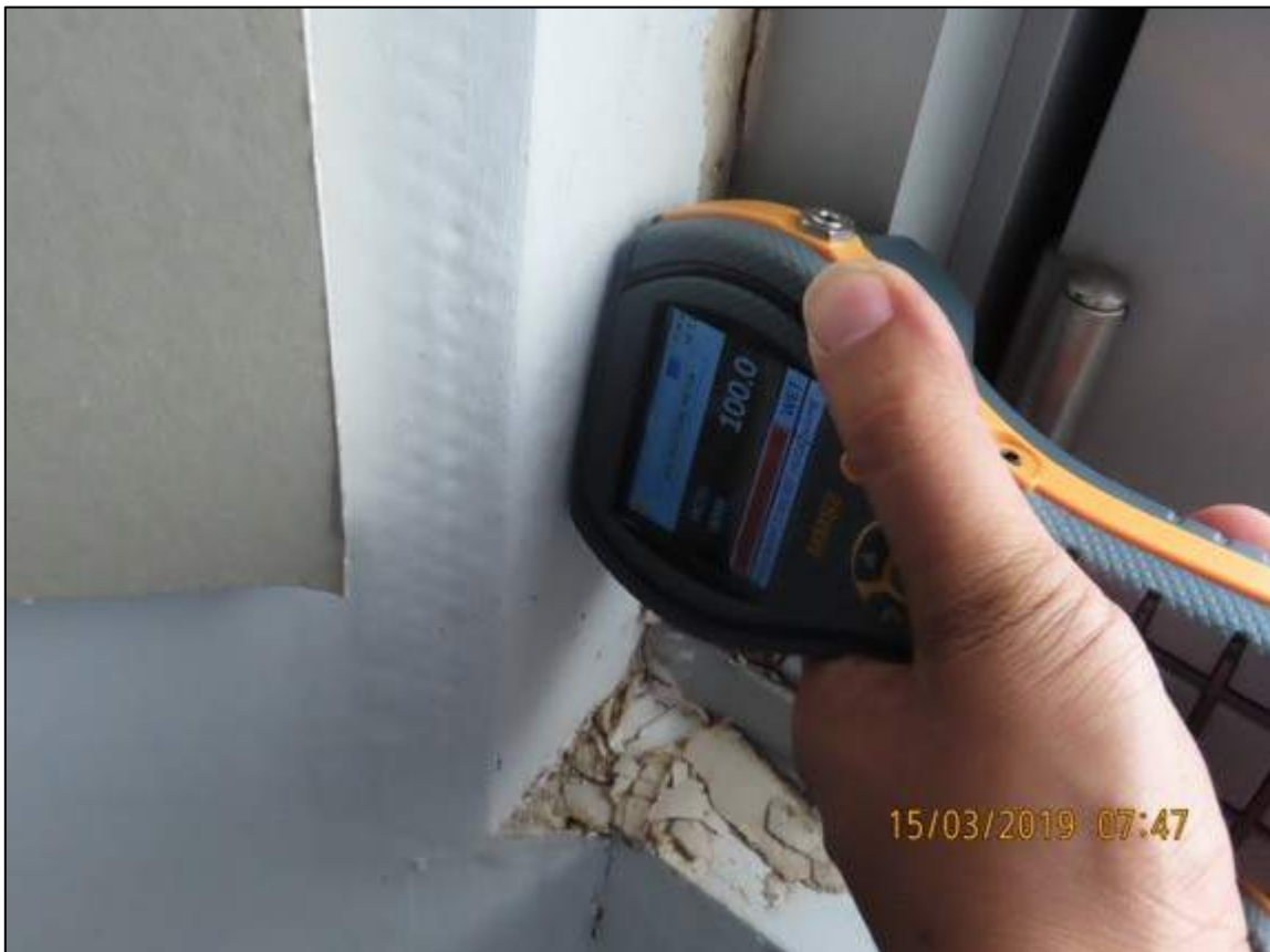
Photograph 29: Showing elevated moisture readings adjacent to Enclosed Balcony windows of Unit 18.
