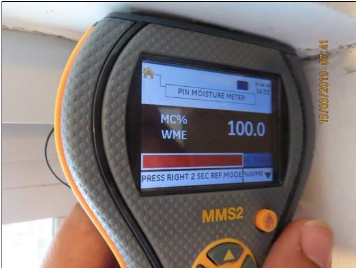
Photograph 36: Showing elevated moisture readings adjacent to Bedroom window of Unit 19.
