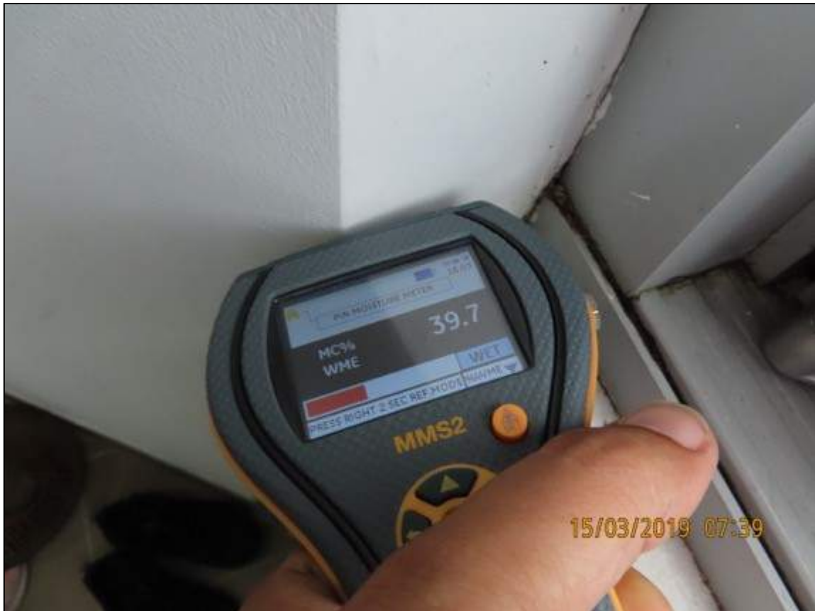
Photograph 32: Showing elevated moisture readings adjacent to Enclosed Balcony windows of Unit 19.
